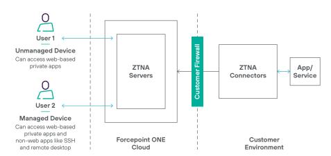
The ZTNA connector initiates an encrypted connection to a corresponding ZTNA server in a nearby Forcepoint ONE local edge data center on AWS. Because the connection is initiated by the ZTNA connector, no inbound ports need to be opened in the private data center firewall.
