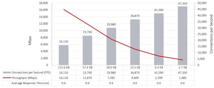
Figure 15 - HTTP Capacity (Clear Text)
