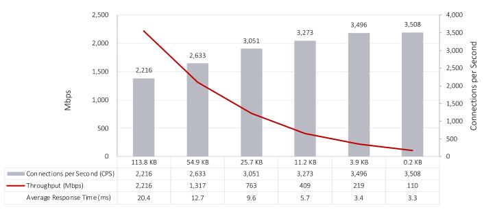
Figure 19 – HTTPS Capacity [TLS\_AES\_128\_GCM\_SHA256 (0x13, 0x01)]
