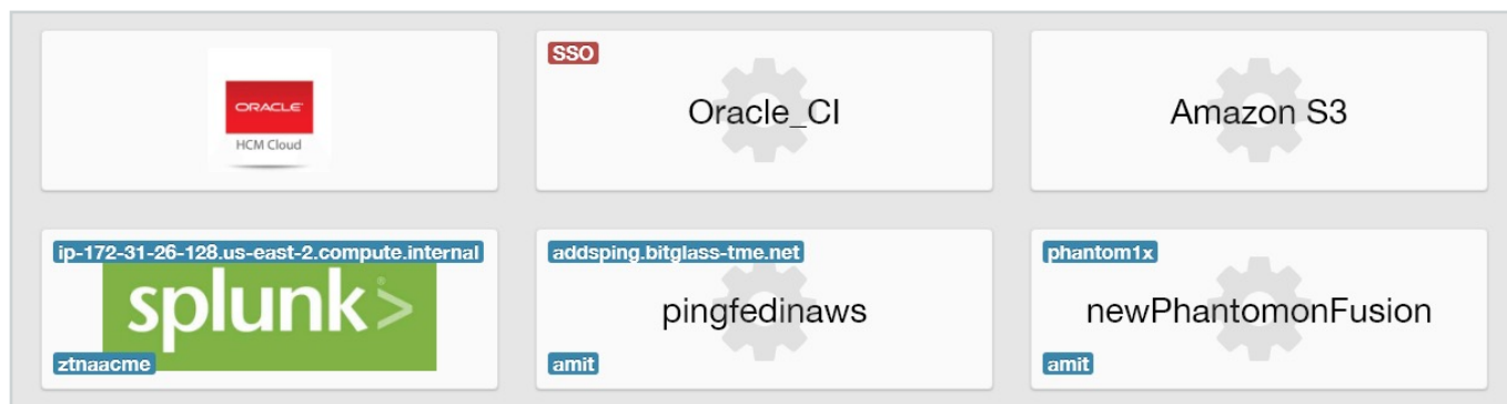
Figure 2: Forcepoint ONE user portal showing both managed SaaS (top) and private web apps (bottom).
